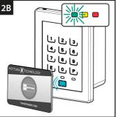
Activate the unit. Press E, digit the ma- Digit a code which become master To add a TAG, show the unknown TAG ster code confirming with E or show and press P, a double flash YELLOW to the reader, a GREEN flash confirms the master TAG. Press E once to enter and GREEN will indicate to re-digit the the operation. same code and press P.
