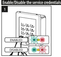
Activate the unit. Press E, digit the master code confirming with E or show a master TAG. Press E 4 times to enter the menu.
