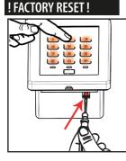
Keep pressed the programming button with a dedicated tool (screwdriver) and activate the unit pressing any other key.
