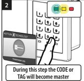
Press any button to activate the unit. Show TAG or digit a CODE 3 to 8 digits. press button P to confirm. Digit again the same CODE or show the same TAG and press P.
