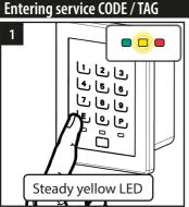
Activate the unit. To enter in program- Digit a code for service and press P, a Show the unknown TAG to the reader, ming press E, enter the master code double flash YELLOW will indicate to the GREEN flash will indicate the corconfirming with E or show a master enter the same code and press P. TAG.
